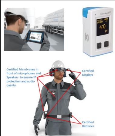
Fig. 21: Mobile devices as workers equipments and batteries intended for use in environments as defined in 2014/34/EU (ATEX)
