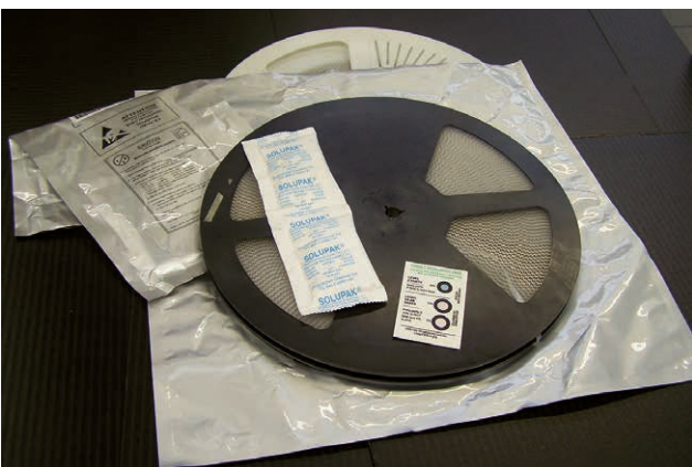
Component-rolls with moisture barrier bag, moisture guard and moisture indicator
