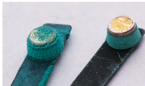
Example of corrosion on an electrical contact
