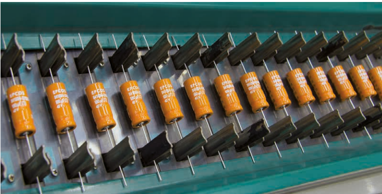
Production of aluminium-electrolyte-capacitors
