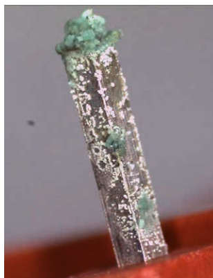
Example of corrosion on a pin
