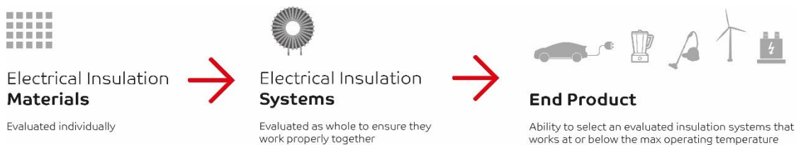
Illustration 4: Process flow: From material to end product approval, image source Synflex
