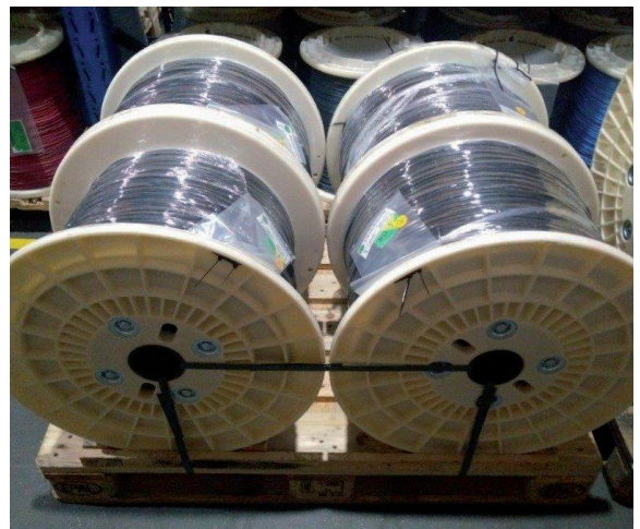
Fig. 8: Reel placed upright on its flange
